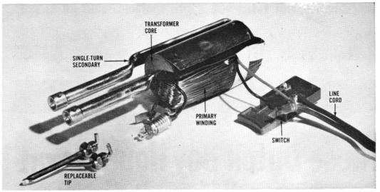
Coiled, flat ribbon of iron makes transformer core. To wind laminations through preformed wire coil, Weller invented a production machine. Real secret of gun's performance is copper-tubing secondary winding. It not only conducts heavy current without overheating, but acts as heat sink to cool upper end of hairpin tip and thus concentrate heat at soldering peen.
