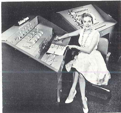
SOLITROL Lighting Control System for theatres, schools and TV Studios was first introduced in 1961 at the American Educational Theatre Association's Silver Anniversary Convention, Waldorf-Astoria, N. Y. The master and preset consoles shown remotely control the solid state dimmers.
