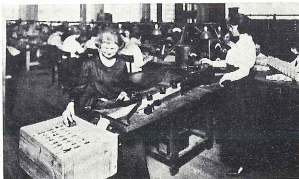
1921—Automatic cut-outs for automobile battery-generator systems undergoing assembly and test. Manufacture was later discontinued when major auto makers produced their own devices.
