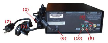
mation). To connect to your television or monitor, you have to verify what type of connection your TV has. Most TV's and monitors have a "Composite Video" input. This connector is typically yellow. You can use the included cable (3) to connect the yellow jack of the DVD player (8) to the yellow jack of your TV. The other 2 connectors on the cable we sent you are for right and left audio. Simply use the red RCA on the cable and
