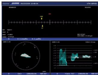
MULTI Mode Display showing Relative Timing with Waveform and Vector.
