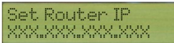
When the "ROUTER IP" option is selected, the top line of the LCD will read "Set Router IP" and the bottom line will display the IP address in the format of "XXX.XXX.XXX.XXX" with the first "X" of the first set blinking
