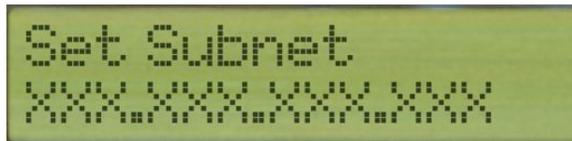
When the "SUBNET" option is selected, the top line of the LCD will read "Set Subnet" and the bottom line will display the IP address in the format of "XXX.XXX.XXX.XXX" with the first "X" of the first set blinking
