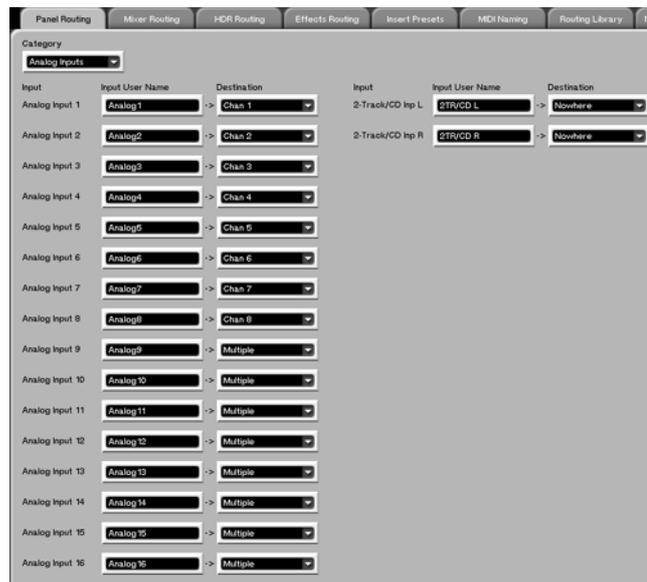
In the **MAIN DISPLAY MODE** area, press the **ROUTING** key to recall the ROUTING SVGA screen.
