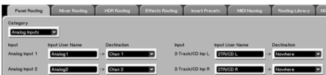
**Category** Selects between viewing the routings for: Analog Inputs, Outputs, Digital I/O, and Option Slots 1-3.
