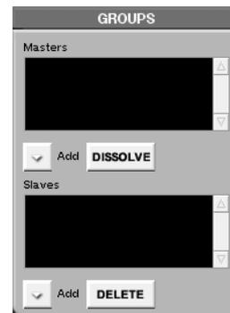
**Masters** This window displays the master faders associated with the selected channel.
