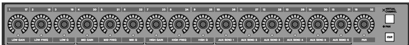
The knobs at the top of the channel strips (above the faders) are multi-function, infinitely rotating potentiometers (pots for short).
