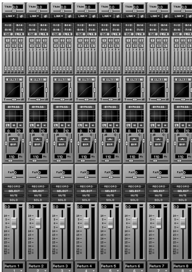
Master levels for the Aux Returns are reached through the Fader Banks. To see the return levels on the SVGA, make sure the Mixer screen is selected (press **MIX** in the **MAIN DISPLAY MODE**). From the **FADER BANK** section, press **BANK MODE** so that the **<PRESET>** LED is on. Then press **RTN/ GRP** to reach this screen.
