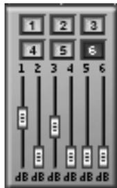
Aux send levels can be controlled from the SVGA Channel screen in the AUX SEND module and from the LCD MIXER CHANNEL page. Identical controls (pictured left) are also found on the channels in the Mixer screen. As well, all 6 Aux Sends are also part of the Virtual Channel Strip for each channel.
