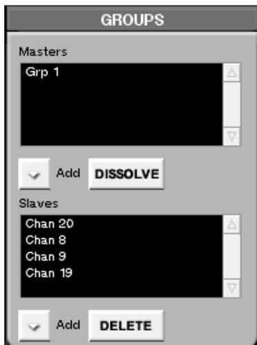
Press **CHANNEL** in the **MAIN DISPLAY MODES** section to find this module. From here you can add and delete master and slave faders.
