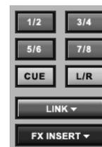
**Bus Masters** Master levels for the busses are reached through the Fader Banks. To see the busses on the SVGA, make sure the Mixer screen is selected (press **MIX** in the **MAIN DISPLAY MODE**). From the **FADER BANK** section, press **BANK MODE** so that the **<PRESET>** LED is on. Then press **BUSS/AUX** to reach this screen.
