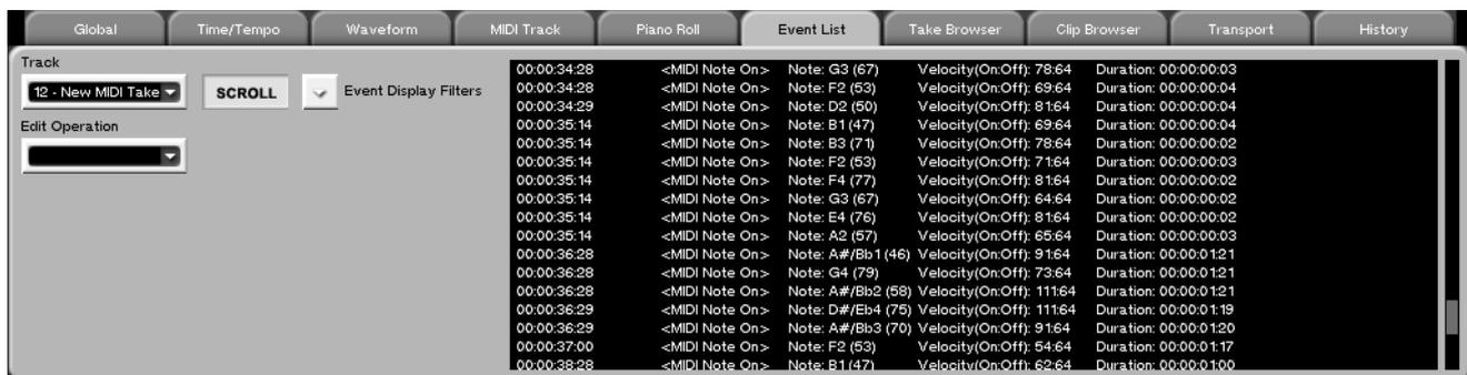
From the AUTOMATION screen, click on the Event List tab. Here you can see the automation events for specific controllers of a selected channel or effect plug-in. It is also possible to edit automation data from this tab.
