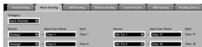
**Category** Selects between viewing the routings for: Input Channels, Aux Returns, Direct Outs, Bypass, Loopback, and Busses.
