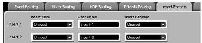
**Insert Send** This field determines where the insert send goes. Notice that external ports are available, making external inserts possible.
