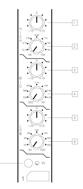
Figure 10. Equalizer Channel
