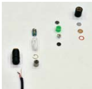
The internal structure of the UWP-V1 lavalier microphone – a new design providing better sound quality.
