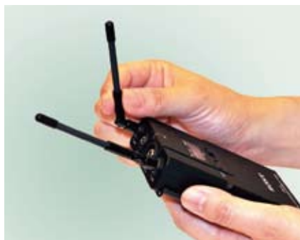
Receiving antennas are designed for easy mounting on camcorders.
