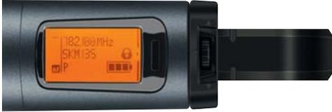
Next to the display - just above the transmitter antenna - is a small wheel. This wheel is used to change and adjust levels and the parameters of the transmitter. Please note that the microphone is suited with a protection ring (available in different colours) to avoid changes caused by non-intentionally pressing the control buttons. If necessary turn the ring to uncover the wheel, making changes possible.
