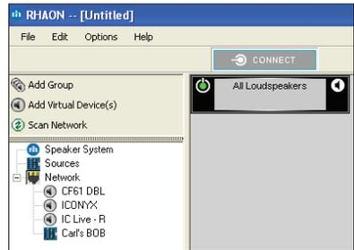
Use your mouse to drag the array listing into the work space where it will show up as an icon. The Status Bar at the bottom of the icon will be red while the array is being synced and then turn green. It will also turn red whenever the program detects a problem with the associated array. Double clicking on the icon will open that array's Connect Properties window.
