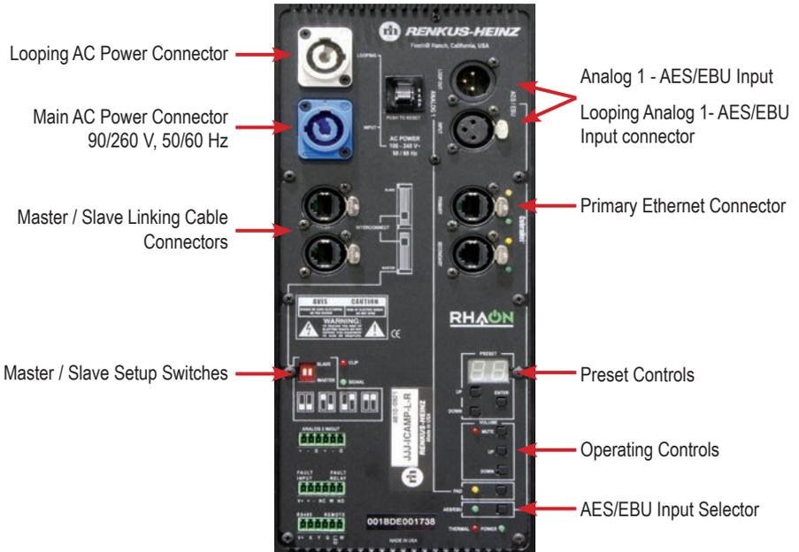
Note: If you are working with a stacked array and one or two subwoofers, make sure your power source (power strip) is adequate to handle the power drain. A stacked array will draw up to 13 Amps at 120 Volts and each IC215S-R needs a 15 Amp source.
