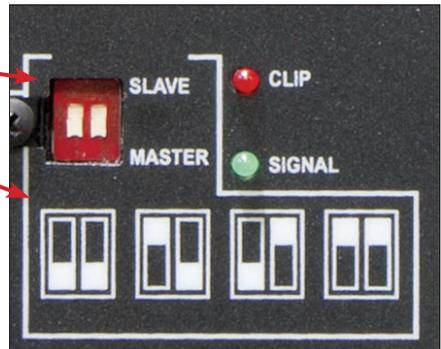
Note: If you connected power to the array before setting the dip switches, you will need to disconnect it and then reconnect it before the dip switch settings will take effect.
