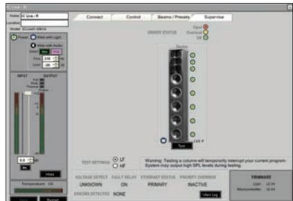
The usual method of monitoring a multi-array system during a program is to watch the array icons in the work space. Green status bars mean everything is fine, yellow bars indicate the array is being overdriven and red bars indicate a problem has been detected. Double clicking on that array's icon will open its supervisory window and provide more details on the problem.
