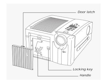
Remove the lamp assembly Unlock the lamp assembly by rotating the locking key on the right side of the lamp assembly counter-clockwise onehalf revolution. Grasp the wire handle and gently pull the lamp assembly straight out of the unit.
