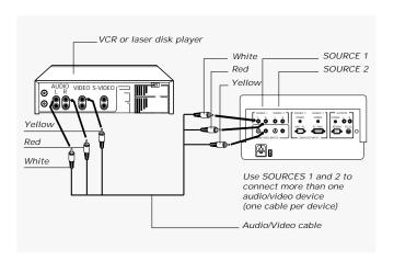
The projector is also compatible with S-video sources (for the appropriate connections, refer to the illustration on the next page).
