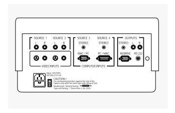
3 You can simultaneously view your desktop computer monitor and project computer images with the projector by connecting your monitor to the REDRIVE port on the rear panel OUTPUTS section. (Refer to the applicable setup procedure in Chapter 3, Detailed setup to connect your monitor.)
