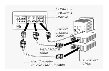
2 If you want to be able to view your computer monitor and project images with the projector simultaneously, connect your VGA monitor cable directly to the REDRIVE port on the projector connector panel.
