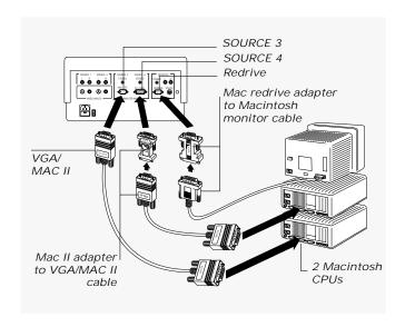
2 If you want to be able to view your computer monitor and project images with the projector simultaneously, connect the Mac monitor redrive adapter (part number AD06) to the REDRIVE port on the projector connector panel and then plug your Macintosh monitor cable into the adapter.
