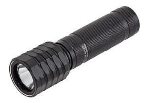
The Mediterranean's fatter lamp contains a three watt Luxeon LED, but the light only runs it at 1.5 watts. It costs \$US109.95, it's about 90mm (3.5 inches) long without key-ring lug, and its quoted CR123 battery life is ten hours - but with only two hours before 50% brightness.
