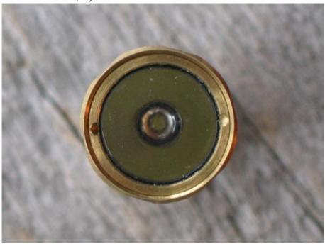
To verify the durability, I dropped the light repeatedly from a height of six feet onto my wooden deck. It was no surprise to find that everything still worked properly. The electronics are potted in epoxy, unlike inexpensive LED lights whose electronics are often susceptible to damage from shock. Don't ask me how I know. This potting also assures that even if water gets by the reliable o-ring seal, it is unlikely that anything (except perhaps the battery) will
