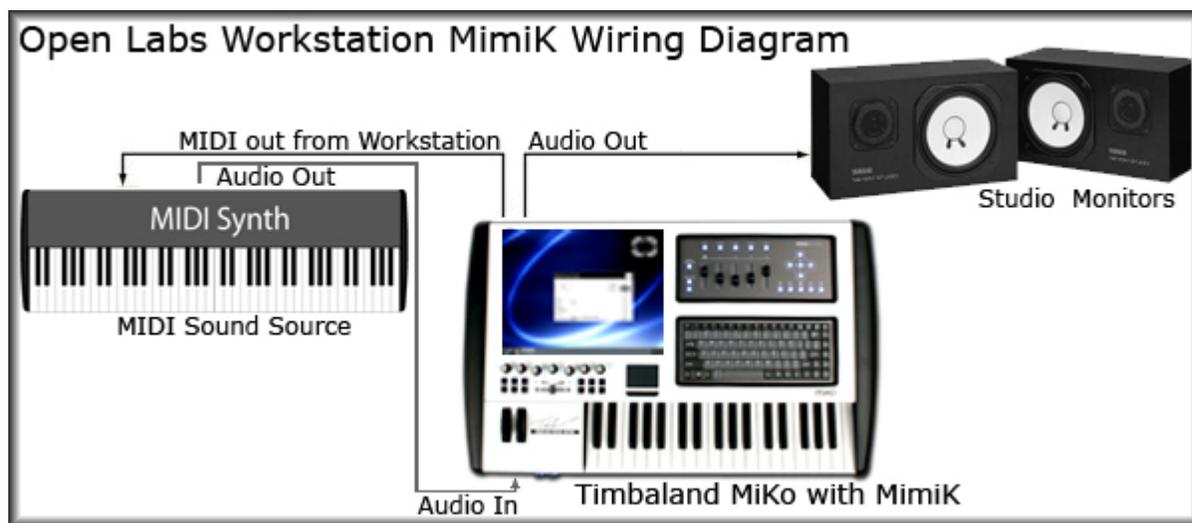
Turn on the keyboard you want to mimic. You will need a standard MIDI cable and one or two ¼-inch audio cables (One audio cable if you want to record in mono, two for stereo).
