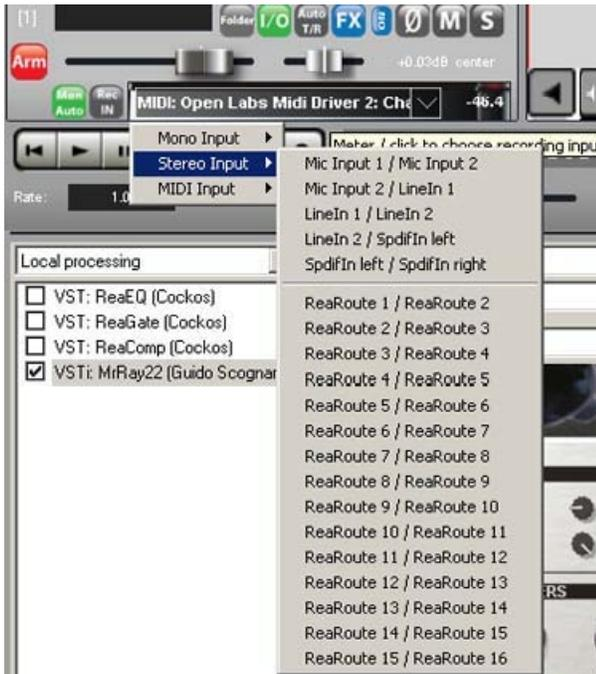
Stereo input allows a source to be assigned to paired inputs of the Firebox. The process is the same as for the mono inputs, except the stereo-ins are paired together as Mic 1 and 2, and LineIn 1 and 2.
