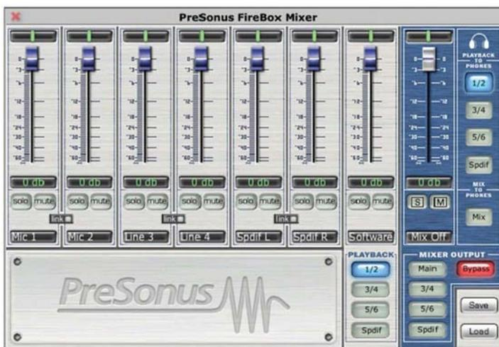
**Note:** The default settings (pictured above) for the interface mixer has all faders set to 0dB and all pans set to center, with the Software Playback set to channels 1/2, the Mixer Output set to Bypass, and the Playback to Phones set to channels 1/2.
