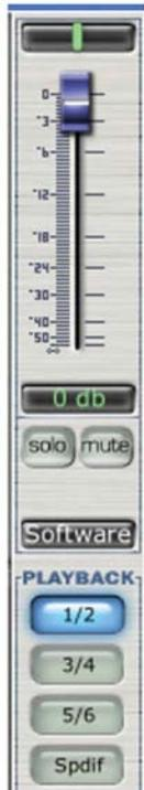
**Input (software playback channel)** – This is the audio return from your audio software. The same functions are available as the other inputs including PAN (balance between left and right channels), LEVEL, SOLO and MUTE. This is a stereo channel. This channel picks up the audio stream that is sent from your software and enables you to mix it with the direct input of your FIREBOX.
