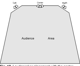
**Fig. 12** Loudspeaker placement with the center loudspeaker forward and raised.
