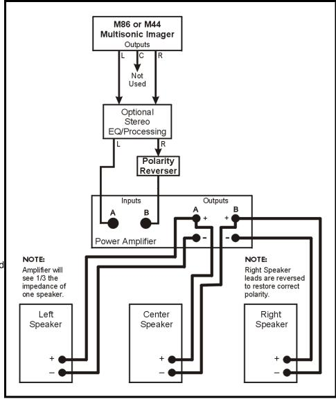
Fig. 15 M86 or M44 Connections with Bridged Center Loudspeaker.
