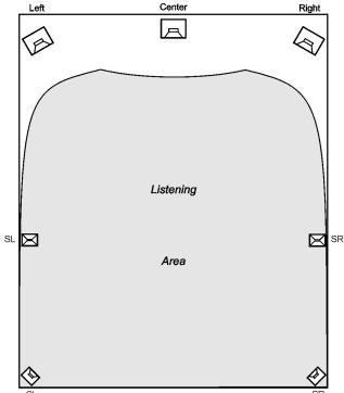
**Fig. 10** Loudspeaker placement for Multisonic Imaging with surround.
