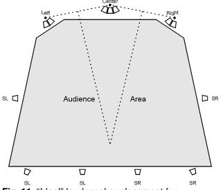
Fig. 11 "Ideal" loudspeaker placement for auditorium.
