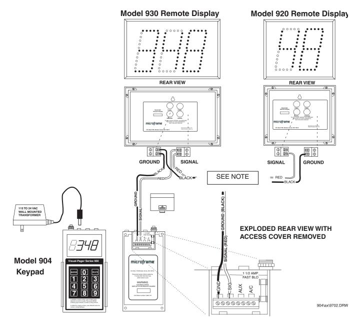
**NOTE:** The Model 920 **SIGNAL** connection is on the Left and **GROUND** is on the Right. On the Model 930, 940 and 960, the **SIGNAL** connection is on the RIGHT and **GROUND** is on the LEFT.
