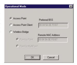
· Access Point Client -A WAP11 set to Access Point Client mode is able to talk to one main WAP11 and wireless clients within its range. This mode allows your WAP11 to act as a client of a main WAP11. A LAN attached to your WAP11 client can then be wirelessly bridged to the main WAP11. Enter the required MAC address of the main WAP11.
