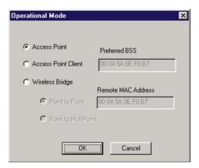
Access Point Client -A WAP11 set to Access Point Client mode is able to talk to one main WAP11 and wireless clients within its range. This mode allows your WAP11 to act as a client of a main WAP11. A LAN attached to your WAP11 client can then be wirelessly bridged to the main WAP11. Enter the required MAC address of the main WAP11.
