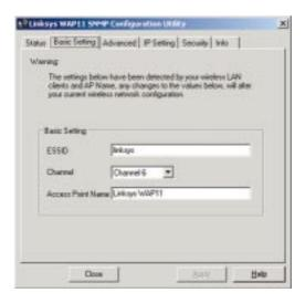
The Wireless Network Access Point will automatically detect the settings to your wireless network. Changing these values will alter your current wireless network configuration.
