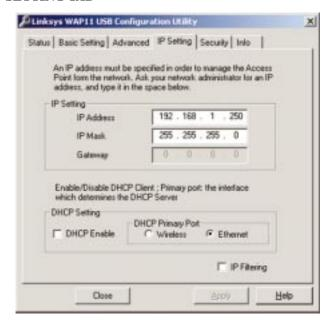
The IP settings for the Wireless Network Access Point are made from this tab.
