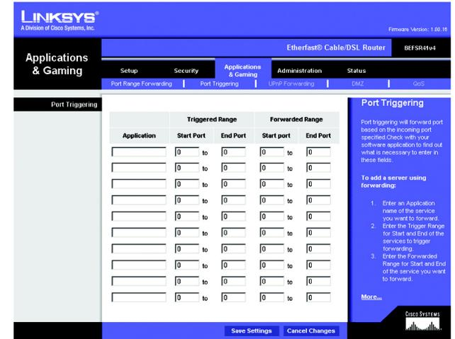
Figure 5-19: Applications & Gaming Tab - Port Triggering
