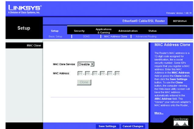
Figure 5-12: Setup Tab - MAC Address Clone
