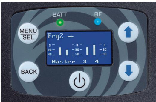
The blue "RF" LED indicates an RF lock between the transmitter and receiver, when lit.
