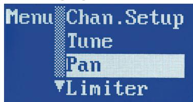
Press the **MENU/SEL** button to enter the setup screen. The setup screen that appears will be determined by the 2 channel or 4 channel mode and the knob configuration you have selected. Continue pressing **MENU/SEL** to select the channel, then use the **UP** and **DOWN** arrows buttons to adjust the balance.
