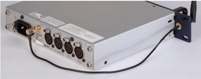
9. Attach the supplied antenna connector protectors to the sides of the transmitters right behind the rack ears. Secure them with the supplied screws. Note that this item will fit tightly and is meant to deform slightly during installation.
