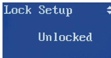
To return to the unlocked status, go back to the **Lock Setup** screen via the main menu, and select **Unlocked**. Also, note that the **Locked** status is maintained even if the batteries are changed.
