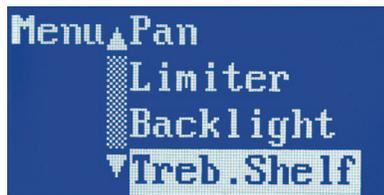
This high-frequency boost should be used sparingly due to the fact that it can accelerate hearing loss with high volumes in the earphones or headphones. Note: the factory default setting is 5 kHz corner with 0dB boost.
