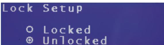
NOTE: Features not affected by **Lock Setup** include channel monitoring selection and headphone volume.
