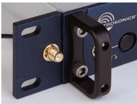
3. Insert the rack ears and attach the handle to the front of the panels using the supplied hex-head bolts and hex wrench. The screws should go through the handles, through the front panel, and into the rack ear nuts. Tighten these bolts loosely.
