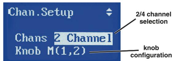
Press **MENU/SEL** to toggle the highlight between the **Chans** and **Knob** lines and use the **UP** and **DOWN** arrow keys to make selections.
