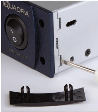
Plastic guards snap out from corners. Pry out the aluminum inserts on the side panel with a small screwdriver.
