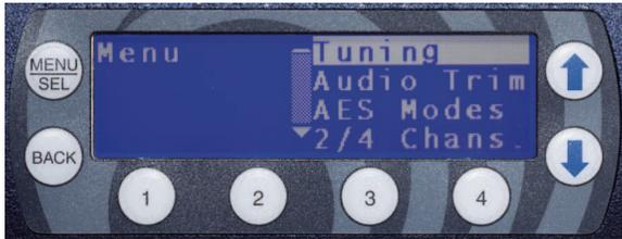
When the desired menu item is highlighted, press the **MENU/SEL** button to enter the setup screen.
