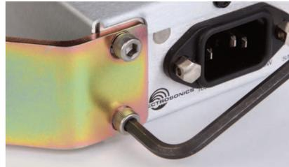
7. Attach the steel brace to the blank panel using the supplied screws. Tighten all four screws that retain the brace.
