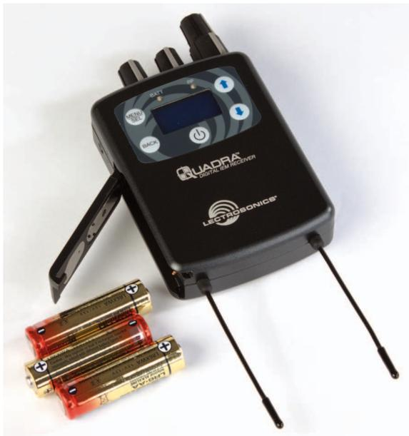
Once the three batteries are in place, close the door by swinging it shut then sliding it upwards while applying slight pressure. It should snap shut and line up with the case.
