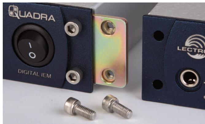
**NOTE:** The threads in the front adapter plate are a self-locking type. Tighten the screws until the head is flush with the front panel.
