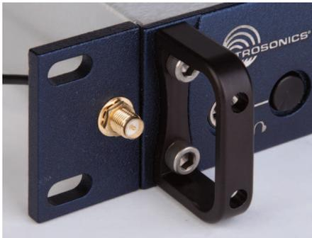
4. Attach front bracket plate to right side of panel.
