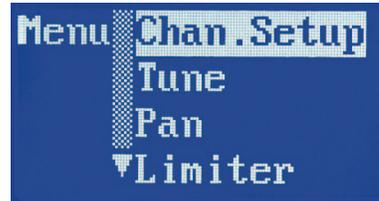
Each **Chan. Setup** screen allows selection of 2 Channel and 4 Channel modes, plus a second line for selection of the knob configurations.
