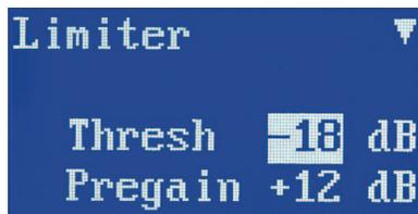
Use the arrow keys to select the limiter threshold in 3 dB increments. Test it with a known signal to determine the maximum sound level you are comfortable with. The pre-gain setting can then be used to boost the audio level ahead of the limiter. Use this feature if you need to make up for weaker audio input levels at the transmitter. Use the **MENU/SEL** button to choose “Pregain”, then use the arrow buttons to adjust in 3 dB increments.
