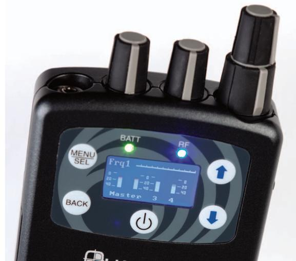
The headphone jack is a standard 1/8” stereo TRS (tip, ring, sleeve) jack with standard headphone wiring (tip is left, ring is right, sleeve is ground). The headphone amp can deliver 100mW into a 32 Ohm load so it is important to always start with the volume low before plugging in your headphones or earbuds.
