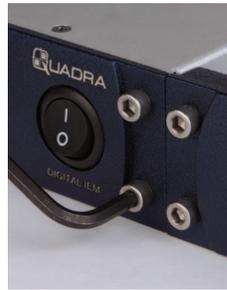
The threads in the front adapter plate are a self-locking type. Tighten the screws until the heads are flush with the front panel.
