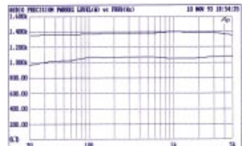
Upper curve shows the LAB 2002 power bandwidth in 4 ohms. US made conventional unit below.
