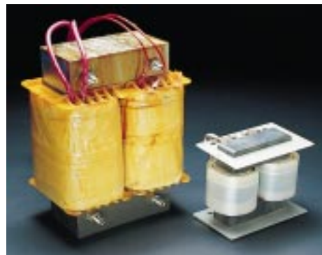
Transformer core made of ferrite, used in the Lab.gruppen switch mode amplifiers, compared with conventional transformer made with iron core.
