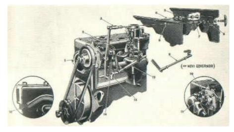
FIG. 34—GOVERNOR INSTALLATION AND ADJUSTMENT
