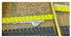
When removing these units from the piano it is perfectly okay to use the gray wires to pull them out of the piano. These wires are very strongly attached inside the sensors and nearly impossible to pull loose.
