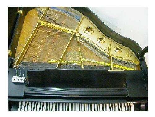
The silver support bars are used to support two sensors under the middle and treble strings. The gold double support bar suspends the third sensor over the bass strings.
