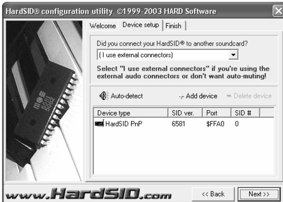
Click "Auto-detect" then click "Start" to re-detect the SID chip on the HardSID PCI, then click "Next" and "Finish".
