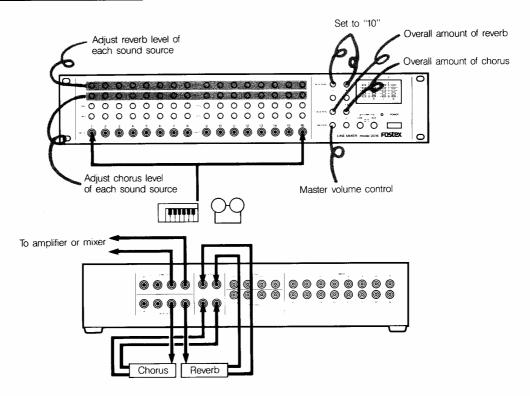
Set the balance of reverb to be applied to the sound sources of each channel by AUX 1 (4) and AUX 3 (7), and also the balance of the chorus by AUX 2 (5) and AUX 4 (8)
