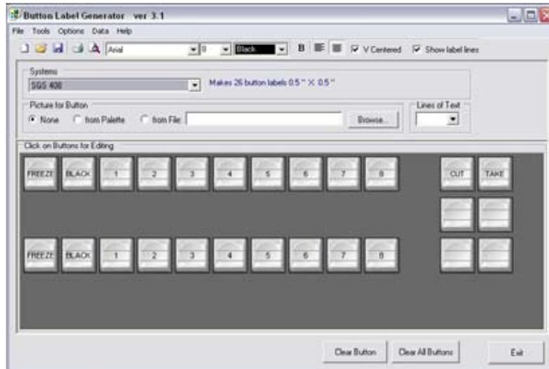
**Figure 5-29 — Extron's Button Label Generator window**
