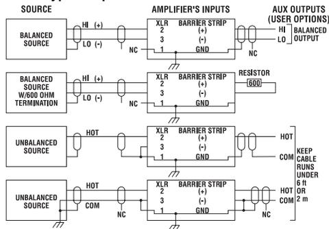
FIGURE 4 — 7100 Typical Output Connections
