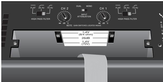
Figure 5.1 Input Sensitivity Switches for CTs 600/1200
