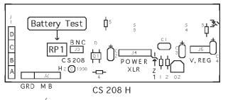
(BOARD H IS INSTALLED ON METER PANEL. REMOVE OUTPUT MODULE TO ACCESS RP1)
