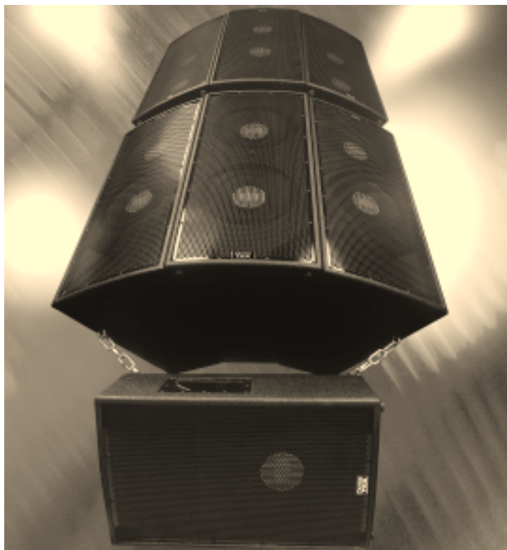
Shown: A typical TCS 60° array consisting of five TCS215's, one TCS215W for bass and one TCS115 mounted at a 45° angle for downfill.
