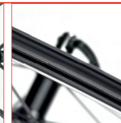
The upper bridge has no spoke holes
