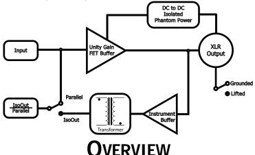
The IsoDI has a transformer isolated power supply to allow a ground lift while still operating with phantom power. Pin 1 on the XLR is always connected to the chassis, but can be connected to the Input ground with the XLR switch.
