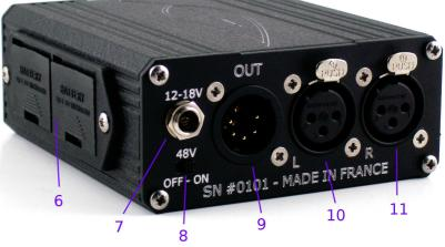
Power socket pinout : Hirose connector pinout : 1 = (-), 4 = (+)Switchcraft connector polarity : inner = (+) , outer = (-)
