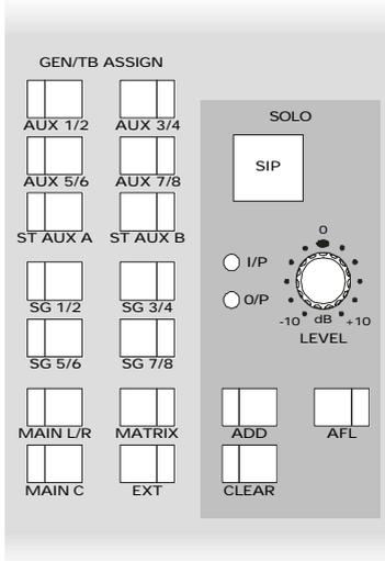
Comprehensive internal assignment of Talkback and Signal generator outputs is provided, along with the ability to send a balanced output to the rear-mounted XLR by depressing the EXT button.
