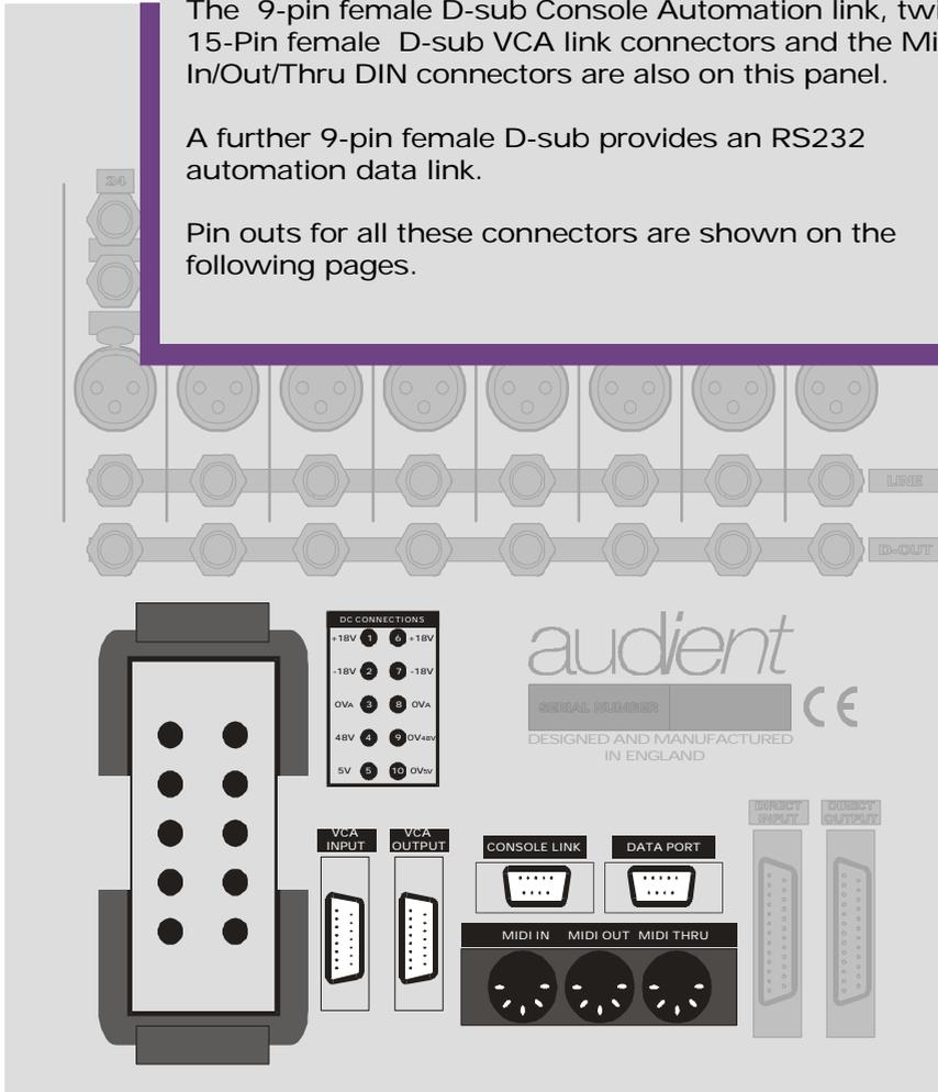
**Connector wiring details - Audio connections**
