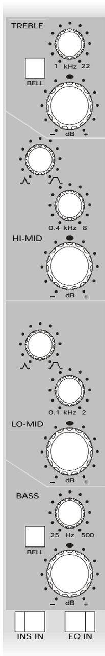
**TREBLE** equaliser with +/-15dB boost and cut variable from 1kHz to 22kHz and selectable bell or shelving characteristics.
