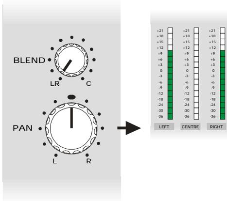
With Blend set in the fully clockwise position only the Centre bus is fed.
