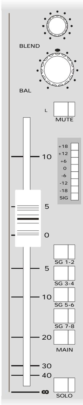
**BLEND** adjusts the relative levels of signals sent to the L/R and C Main buses.
