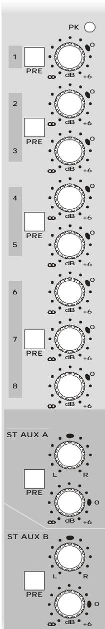
**PK LED** monitors signal levels at mic amp output, insert return and equaliser output warning of levels within 3dB of clip.
