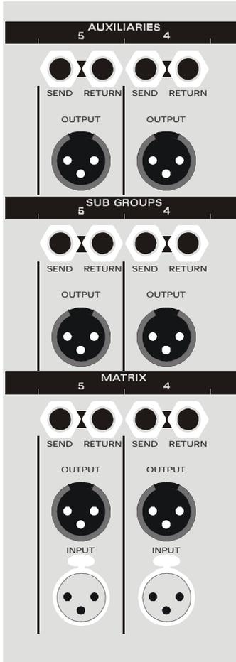
Aztec Sub-Group output module connections are arranged on a single panel along with those for the Master module and Stereo Auxiliary module interfaces.
