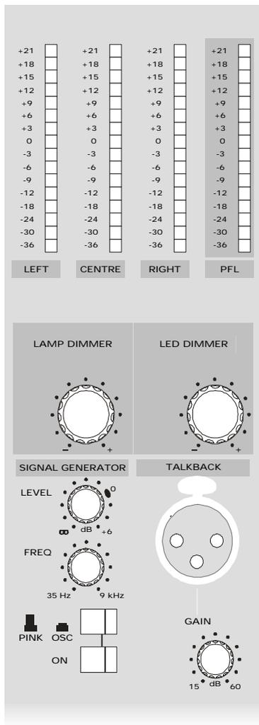
**16 LED** peak-reading meters for the Left, Centre and Right Main outputs.
