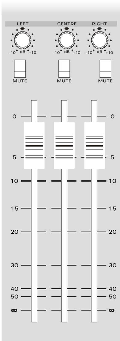
The Main L,C,R outputs are each equipped with a 100mm fader, a **MUTE** and a **TRIM** control providing an additional +/- 10dB of gain adjustment. The TRIM feature allows the faders to always be operated at the desired position without having to use them to adjust L/C/R balance.
