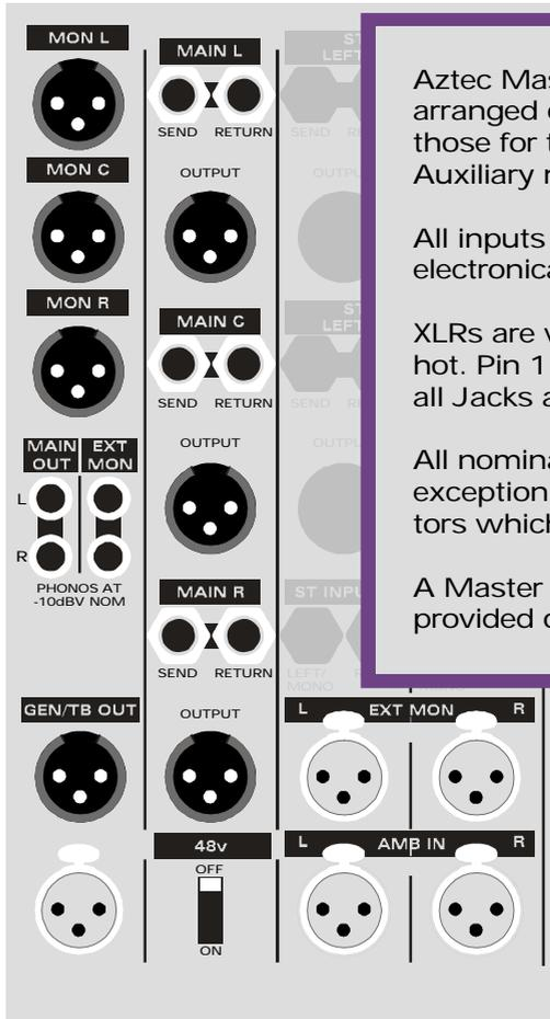
Aztec Master module interfaces are arranged on a central panel along with those for the Sub-Group and Stereo Auxiliary modules.
