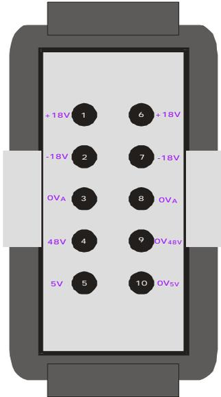
Aztec PSU connector viewed from mating side of console mounted chassis connector.
