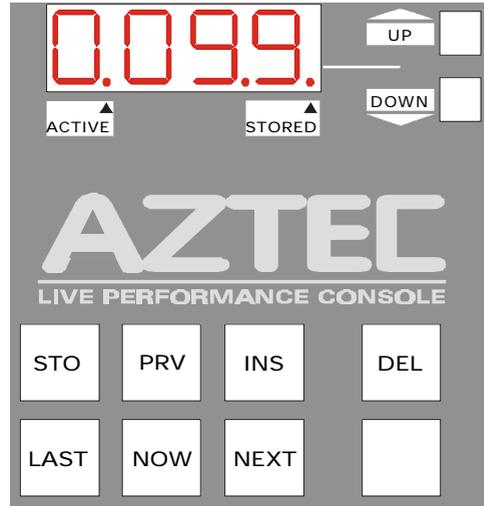
To over-write the existing stored Scene depress STO and hold it down for ~ 2 seconds until the display stops flashing.
