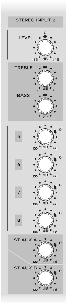
Two identical, general purpose, fully balanced Stereo inputs are provided (only one is shown here).
