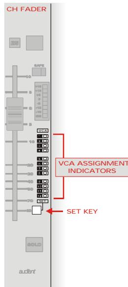
Once the MIDI channel number has been selected, depressing the Input channel SET key will toggle the MIDI message from NOTE ON to NOTE OFF to no message to NOTE ON again. The NOTE setting is shown by the status of channel VCA Assignment indicator LEDs. NOTE ON being indicated by LEDs 1/2 flashing, NOTE OFF by LEDs 11/12 flashing.
