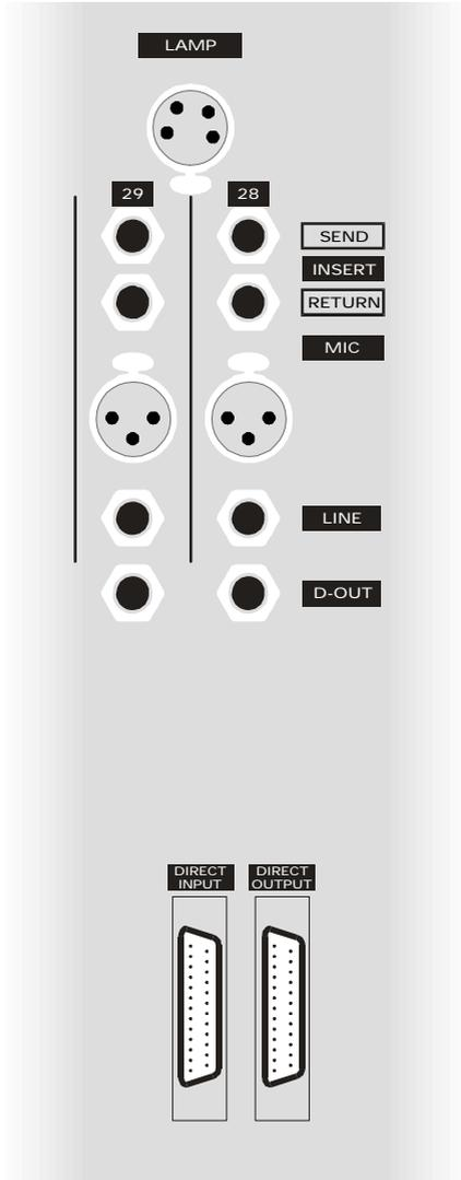
Aztec Input module connector panels are arranged in 8 channel wide panels.
