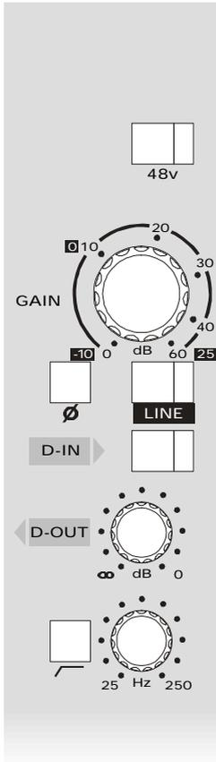
**48v** enables phantom powering. A master isolator is provided on the rear connector panel.
