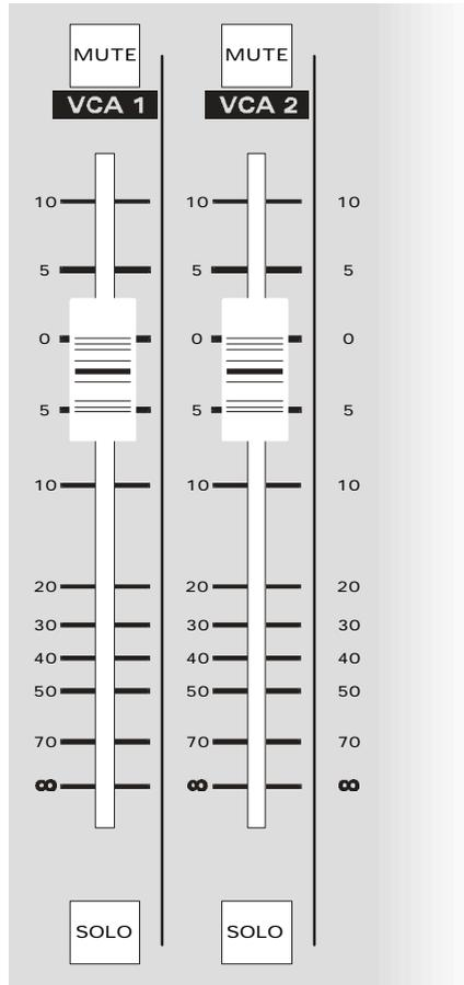
The 12 VCA master faders are fitted centrally in the console fader section below the audio Sub-Group output modules. Each VCA master fader has an associated Mute and Solo switch.
