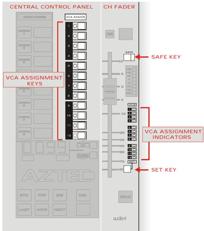
The stored assignment is displayed on the column of 12 LEDs adjacent to each channel fader.
