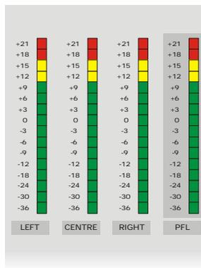
Solo'd AFL signals are metered on the L, C, R Master module LED bargraph displays. PFL has a dedicated bargraph display.
