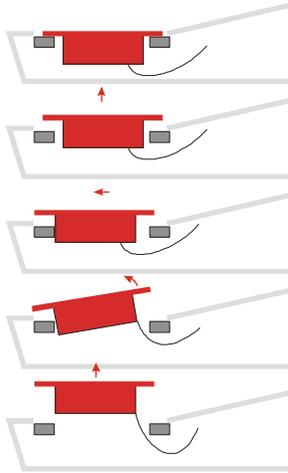
After removing these screws carefully lift the panel by ~20mm then pull it forward slightly being careful to avoid damage to the isolate switch at the front edge of the module.
