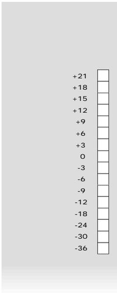
The **16 LED** peak-reading meter can be set to monitor Sub-Group, Auxiliary or Matrix outputs using the **METER SELECT** switches on the adjacent Stereo Auxiliary output module.
