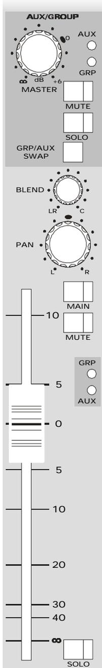
In the default setting the **Auxiliary Master** output level is set using this rotary control with 6dB of gain available. There is an associated automation controlled **MUTE** and a **SOLO** switch.
