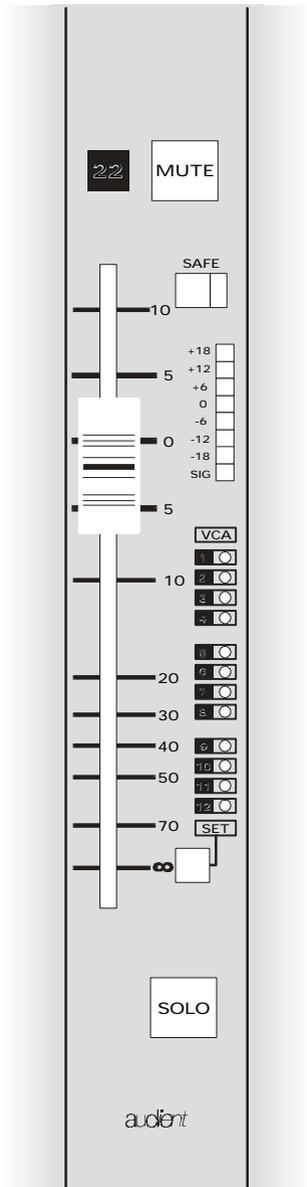
Aztec Input faders are arranged in 8 channel wide panels. There is a single larger panel for the 12 VCA Master faders and the 3 Main Output faders are fitted on the Master output module.
