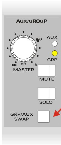
However, when more monitor sends are required the Master level controls for each of the Sub-Group and Auxiliary outputs may be swapped by depressing the GRP/AUX swap buttons on each Sub-Group output module. The function of the rotary control and fader are shown by the LED adjacent to each. The Solo and Mute functions swap with the level control but output connections are unaffected.
