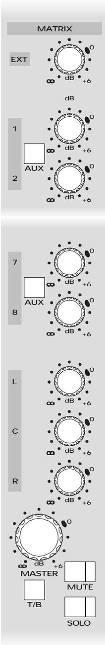
Each of the eight Sub-Group output modules has a 12-way Matrix section.
