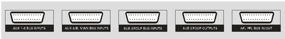
**Stereo Auxiliary module connections**
