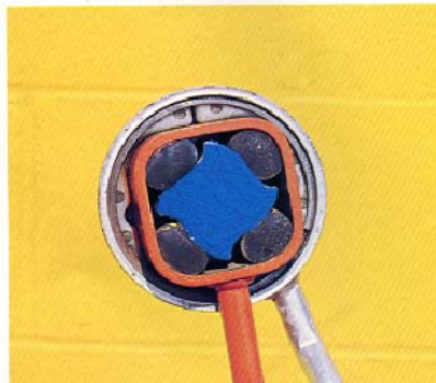
Dura-Torque axle, compressed.
