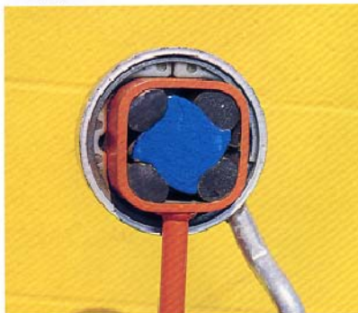
Dura-Torque axle, normal.
