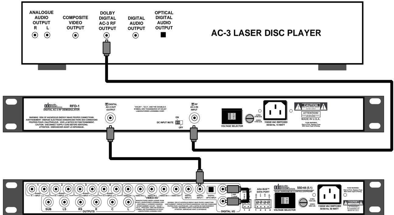
The RFD-1 has a DC Input Mute Switch on its back panel which can be set to either ON or OFF. Normally, on laser disc players with an AC-3 output, DC voltage flows on the AC-3 RF Input and thus the mute switch is left in the ON position. For older laser disc players which have been modified to provide an AC-3 signal, the switch may need to be set to the OFF position.
