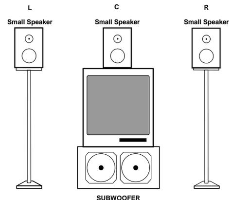
In this option, you will want to engage the 80Hz Cutoff filter for the center channel and the front right and left channels.
