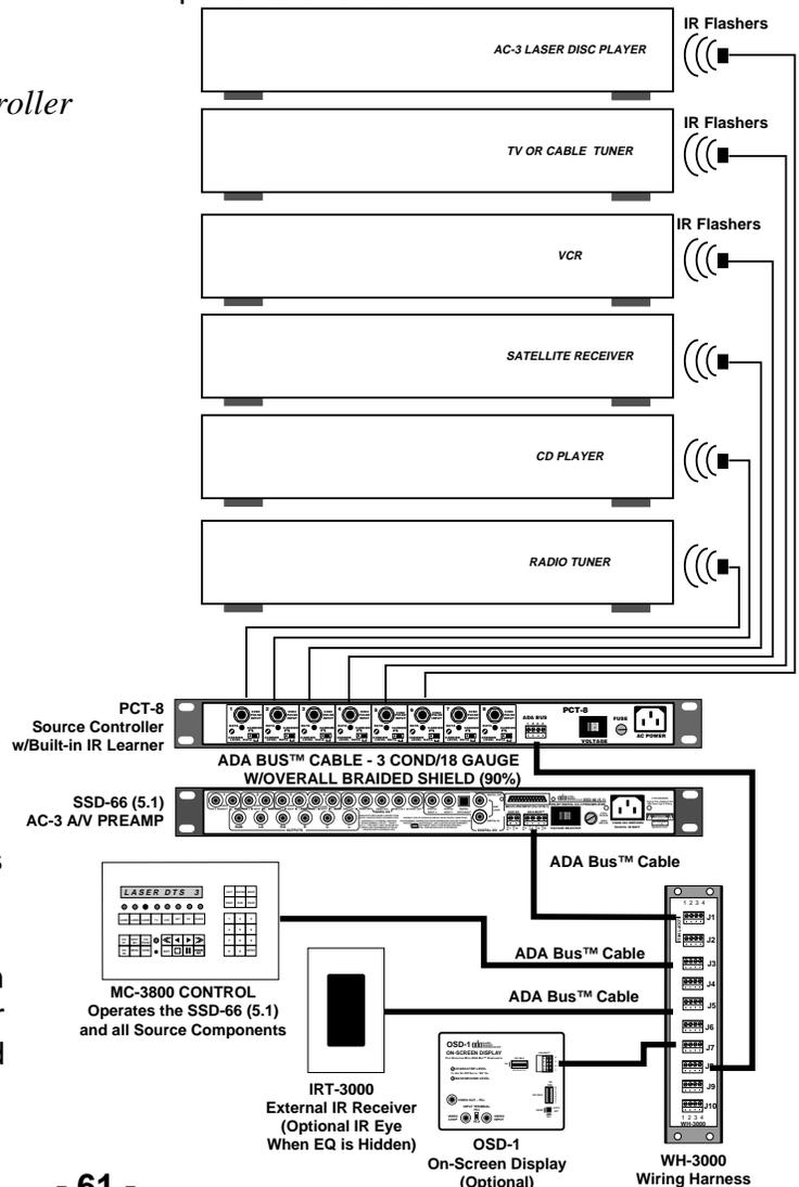
**PCT-8 • IR Learner** capable of controlling up to eight source components (i.e. VCR, Laser Disc Player) and learning 19 functions (i.e. Play, Stop, Pause) for each component (152 total commands). Functions are programmed directly into the PCT-8's front panel IR receiver using the source component's original IR remote control.
