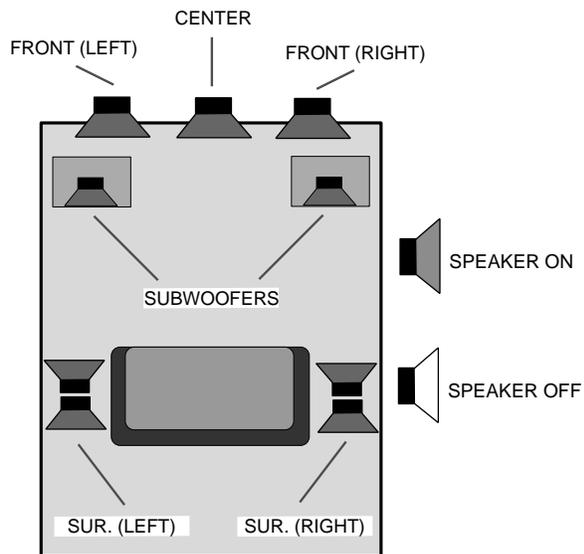
While in the Pro Logic mode, the surround channels will also have a Rear Channel Noise Reduction filter fixed in the on position. This filter is designed to eliminate the higher frequencies by cutting off the bandwidth of the surround channels at 7,500 Hz. Thus, the surround channels in Pro Logic receive a bandwidth of 20 Hz to 7,500 Hz rather than the full audible bandwidth of 20 Hz to 20,000 Hz.
