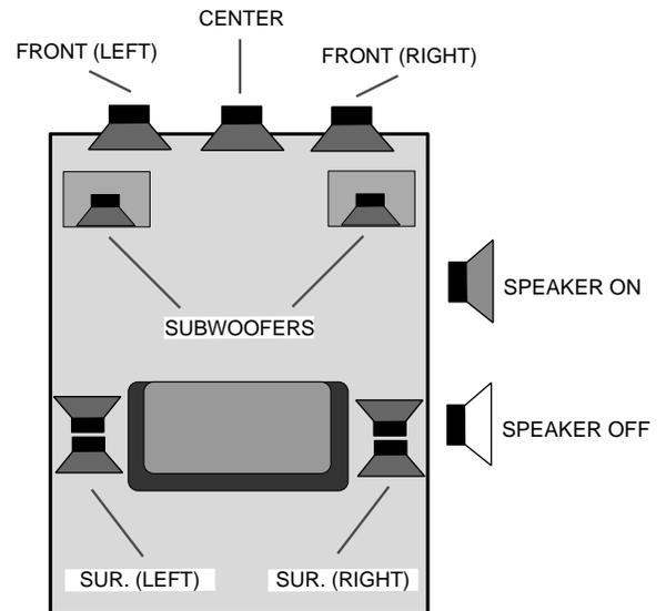
DTS encoded software is very dynamic, especially in the bass channels. Thus special attention needs to be given to the bass summing in that the DTS bass information will most likely need to be toned down approximately 10 dB.
