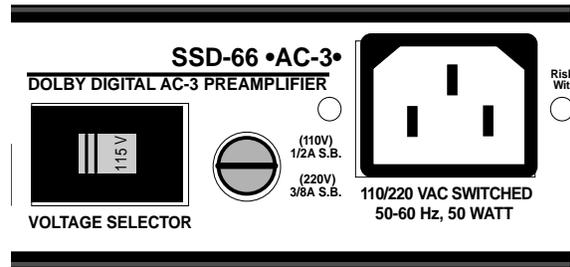
In the United States, the switch needs to be set to the left in the 115V position with a Safety Fuse valued at 1/2 A S.B. In some countries, it will be necessary to set this switch to the right in the 230V position with a Safety Fuse valued at 3/8A S.B. If you are not certain as to which position the "Voltage Selector" switch needs to be set to, consult with your local ADA Dealer.
