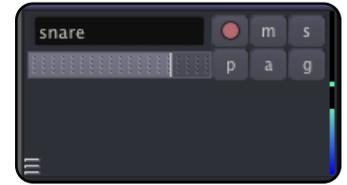
The “P” key on each track allows selection of the track’s playlist. **Playlists** can be used to enable multiple takes in a single track, or the sharing of playlist data across multiple tracks. Some users create a new playlist for each recording “take” while others use **Layers** to manage takes.
