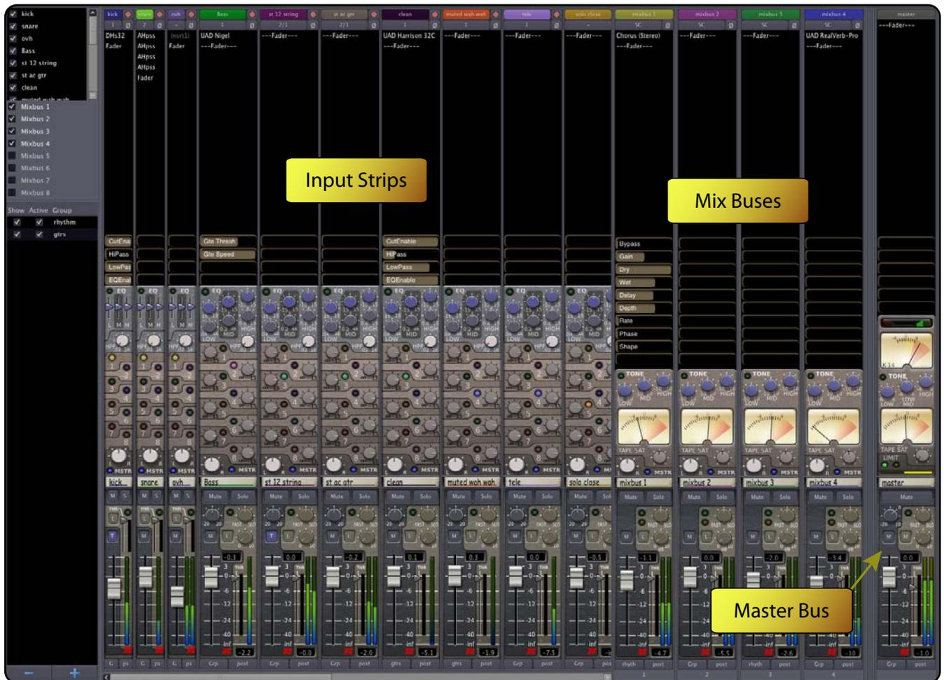
In Mixbus, like other audio workstations, each recording track has its own mixer strip. These mixer strips resemble the input channels of a traditional analog mixing console. Input channels can be configured to be mono or stereo and by default include all the DSP processing that makes up a real console channel. This is the major difference between Mixbus and other DAW mixers. No time is wasted searching for and adding the necessary high-quality mixing tools.
