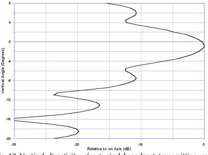
Fig 12 Vertical directivity of a typical broadcast transmitting antenna
