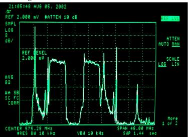
Fig 6. This spectrum analyzer's view of eight UHF TV channels clearly illustrates the nature of the interfering signals that a wireless mic system must compete with. Three analog TV stations and two DTV stations are transmitting in the eight TV channels shown in this scan. Five years ago, those digital transmitters weren't on the air!
