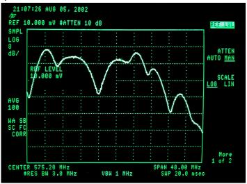
Fig 9 The same eight channels of Fig 6, but with the analyzer bandwidth set to 3 MHz.
