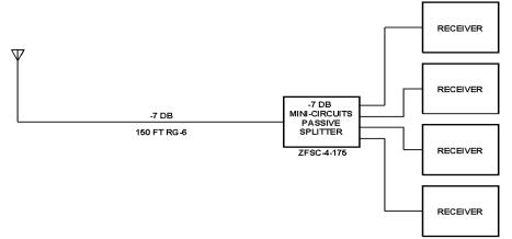
Fig 10 Moving the antenna closer to the talent puts 13 dB more signal at the antenna, but we lose 7 dB in the coax and 7 dB in a passive splitter for a net loss of 1 dB. But any TV interference (including overload or desense that it causes) is reduced by 14 dB!
