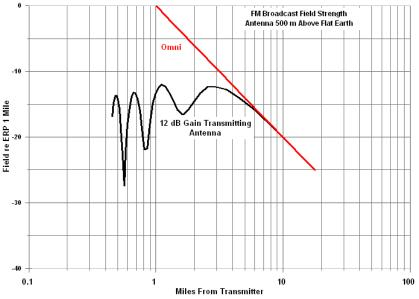
Fig 13 – Field strength on the ground for the antenna of Fig 5 at 500 m
