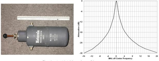
Fig 18 – A 450 MHz cavity and its response
