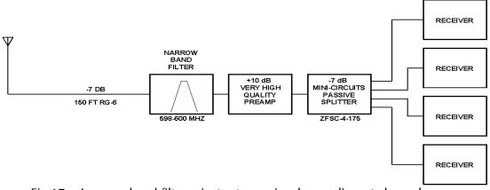
Fig 17 – A narrowband filter rejects strong signals on adjacent channels
