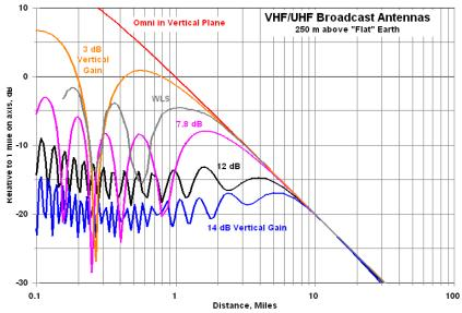
Fig 14 – Field strength on the ground vs. vertical gain for antennas at 250m
