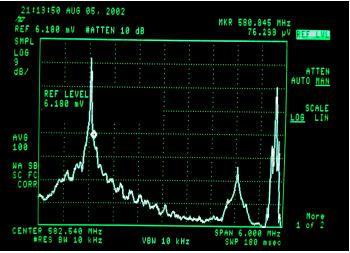
Fig 8. A more detailed view (6 MHz wide) of one of the analog signals. There are two strong spikes (their picture and sound carriers), with energy concentrated relatively close to those carriers. The tall spike at the left of the trace is the video carrier, with most of the power concentrated in sidebands relatively close to it. The tall spike at the right of the trace is the sound carrier. The bump to the left of the sound carrier is the color sub-carrier with its associated energy.
