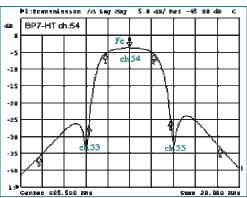
Fig 16 – This larger and more expensive multi-stage filter (about \$450) has both wider bandwidth and better rejection of adjacent transmitters. [The channel identification references CATV channels, not broadcast channels] These filters are from Tin Lee Electronics (www.tinlee.com)
