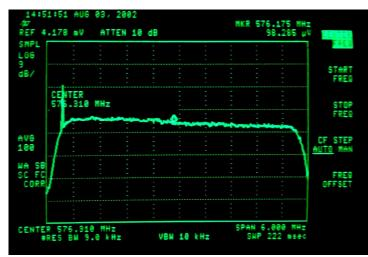
Fig 7. A 6 MHz wide view of one digital TV signal. The digital TV stations (Ch 29 and Ch 31 in Fig 6) show up as a flat trace that exactly fills their assigned channels. The high spike at the left of each DTV station is a pilot signal. Thus the digital station's power is spread equally throughout the channel.
