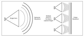
Spherical wavefronts tend to cause interference with adjacent loudspeakers. One common method for "flattening" the wavefront projecting from a vertical line array loudspeaker is to use multiple smaller horns instead of a single horn.
