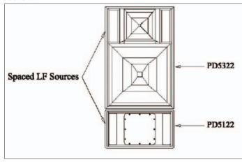
Figure 3 Bipole configuration using point-and-shoot loudspeaker.
