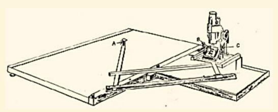
*Fig. 7.* The delineating machine. A, tracing point; B, fingers for clamping the pattern character; C, bed plate showing angle possibilities. Note that the character shown is clamped at an angle, enabling the operator to produce a condensed version of the original. (Redrawn from an illustration in the American Machinist, 16 December 1909.)
