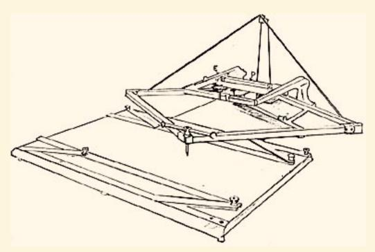
*Fig. 8. The wax-plate delineator. D, tracing point inverted; E, frame for holding plate. (Redrawn from an illus-tration in the American Machinist, 16 December 1909.)*
