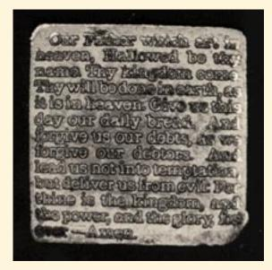
Fig. 6. Microphotograph of the Lord's Prayer cast on the end of an 8-point piece of type. The matrix was cut so that the text would be right-reading. This exhibition of the precision of Benton's matrix engraving machine was used for advertising purposes. (Photo credit, Sheila Donnelley).
