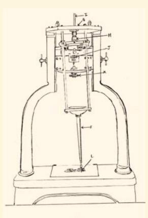
Fig. 9. The matrix engraving machine. F, pendulum; G, yoke; H, quill; I, flexible shaft drive; J, matrix; K, micrometer adjustment; L, follower. (Redrawn from an illustration in the American Machinist, 16 December 1909.)
